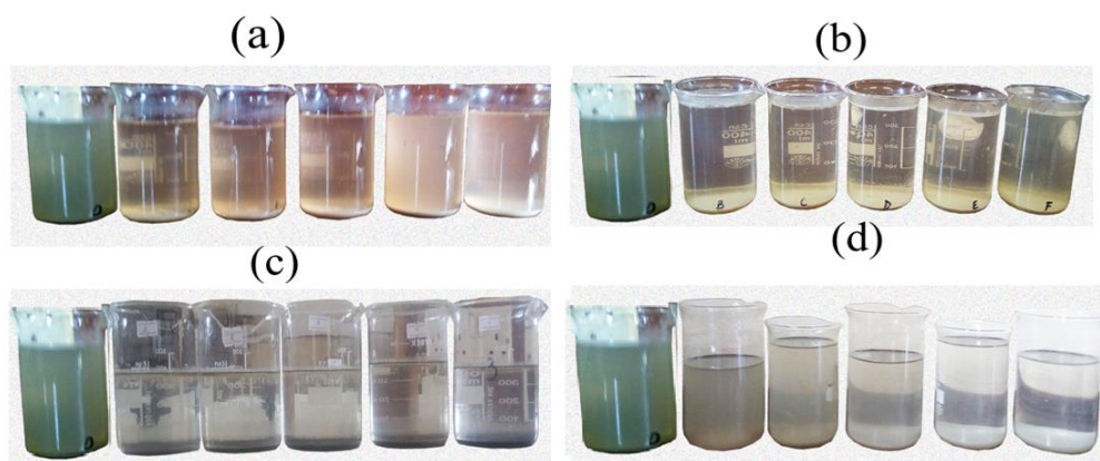
Figure 3: The display of clarified wastewater with different doses of (a) Jatropha curcas (b) Moringa oleifera (c) Rice husks ash and (d) Aluminium sulphate.
